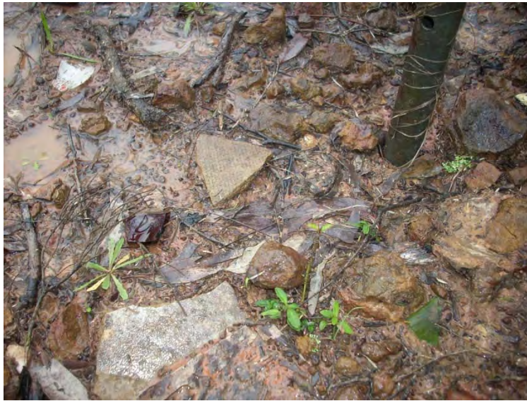
Photo 47. Asbestos containing materials were observed near the sampling location, T2B
